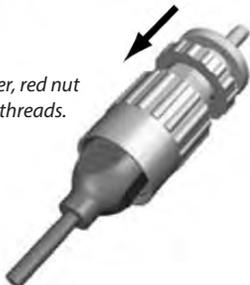
5. Rotate the red nut snugly against the larger nut.
